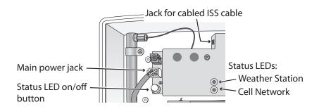
The Vantage Connect will now begin to acquire both the radio signal from the weather station as well as the cell signal. You will be able to observe this by watching the LED lights.
